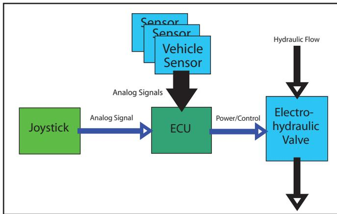
**FIGURE 1: ECU controlling an electrohydraulic valve by processing a joystick command under consideration of other vehicle-sensor inputs**
