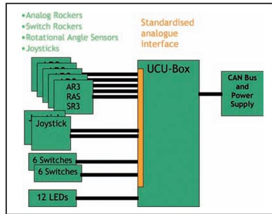
**FIGURE 2: Example topology of an UCU system**
